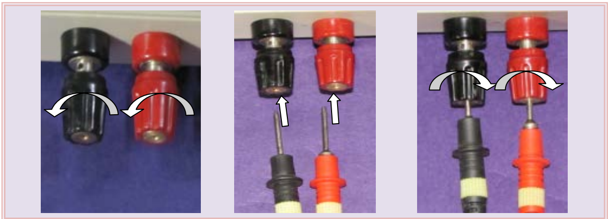
Figure 2A: PSA to Cable connection
