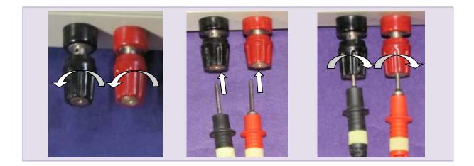
Method : Twist the terminal caps counter clockwise, push the lead electrodes into the end of the collets terminals, tighten the leads by twisting caps clockwise.
